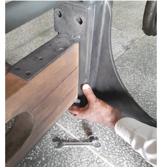
Step 2. Insert the Iron plate making Sure all the holes are aligned.
