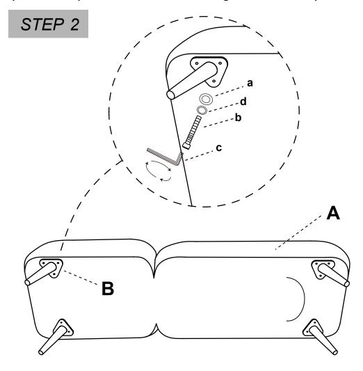
> Use the included hardware to attach the legs to the bench seat as shown.
