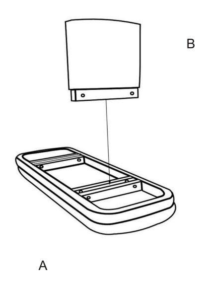
> Insert the top part of the leg in between the supports bar.
