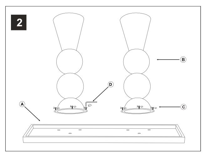
STEP -2: Use the Included Screws ( C ) to attach the base ( B ) to the top ( A )
