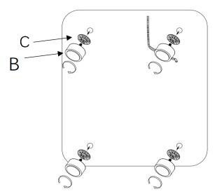
Install the legs by threading them into the pre-drilled holes as illustrated.
