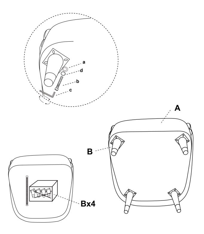
> Position the product bottom-side up and use the included hardware to assemble the legs as shown.
