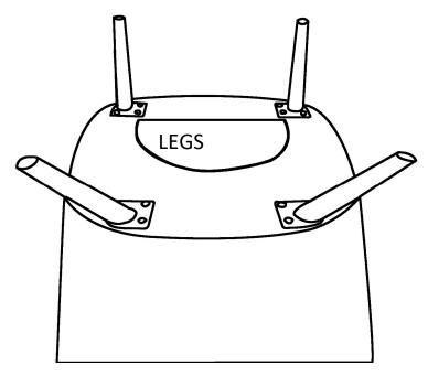
Open the pocket to remove the 4 legs, then close the pocket
