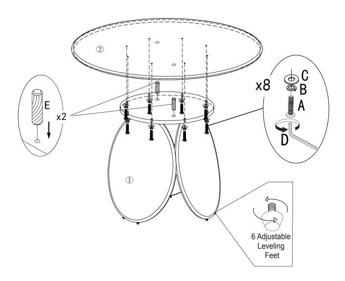
Once the tabletop has been connected to the base, all screws should be fully tightened.
