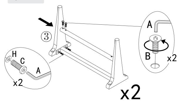
Do not tighten screws all the way at this point
