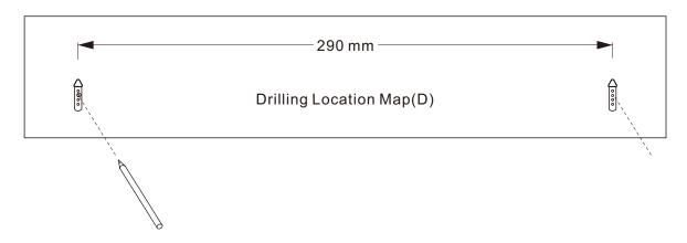
STEP 3: Drill the holes into the wall.
