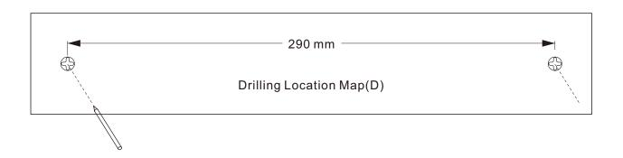
STEP 3: Drill the holes into the wall.
