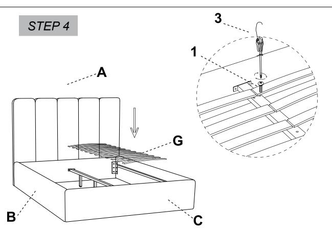
> Screw the bolts (1) into the pre-drilled holes on the support bar to secure the slats in place.
