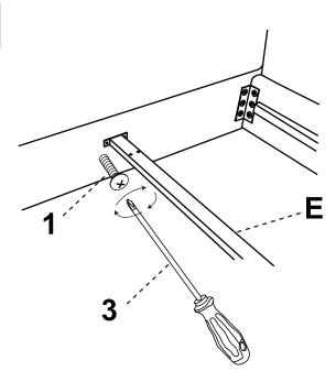
>Attach the center support bar as shown.
