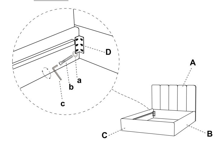
> Using the included hardware, assemble the bed frame as shown.
