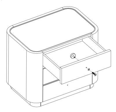
${\sf STEP~2}$  1) Using the same hardware , install the drawer handle as shown.
