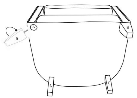
Install Leg into the Chair by Insert the threaded Stem into the threaded Hole at each Corner of the Bottom of the Chair. Tighten by turning Leg clockwise. Repeat the same Step to install the other Leg
