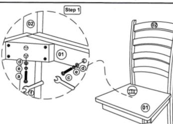
(C1535-RTA) List of Part For 1 Set Qty. Code Figure Part (01) Seat 1 Back Frame (02) 10000 1 03 1 Leg (Left) 1 Leg (Right) 04 Left Side (05) 1 Stretcher (L) Right Side 1 (06 Stretcher (R)
