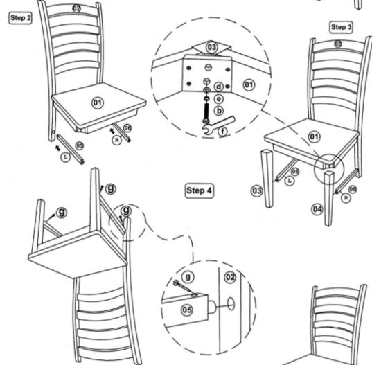
List of hardware For 1 Set Code Figure Hardware Qty. Hex. Bolt 4 0 M6 x 80mm Hex. Bolt 4 Ь M6 x 60mm Hex. Bolt 80 2  $\odot$ M6 x 40mm Flat Washer 10 0 \* x 18mm Spring Washer 0 10 0 5 Spanner 1 1 10mm 9 PHRS Screw 4 #8x11/2"
