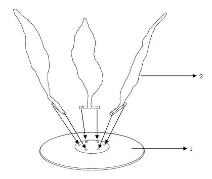
STEP# 2: Tighten the bolts to lock the stretcher as shown below.
