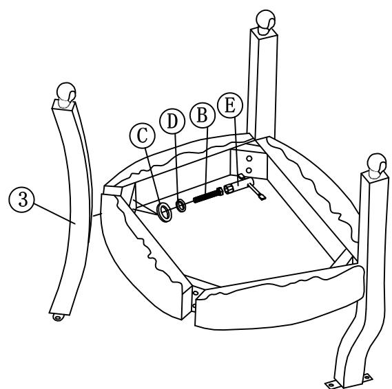
Do not fully tighten the bolts at this step
