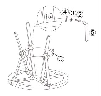
STEP 3: Attach the fourth leg to the Connecting ring (C) and Table Top (A) using Flat Washer (4), Lock Washer (3), Long Bolts (1), Short Bolts (2), Secure by Allen key (5), fully tighten all bolts, at this time. Product assembly is now complete.
