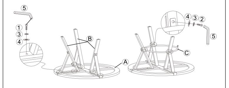
STEP 3: Attach the fourth leg to the Connecting ring (C) and Table Top (A) using Flat Washer (4), Lock Washer (3), Long Bolts (1), Short Bolts (2), Secure by Allen key (5), fully tighten all bolts, at this time. Product assembly is now complete.
