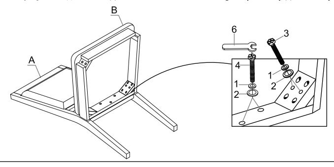
Step 1: Attach Front Leg (C) to the Seat Box W/ Cushion Seat (B) by using Flat Washer (2), Spring Washer (1), Hex Nut (5), secure by Wrench (6). Fully tighten all bolts at this time. Assembly product is now complete.
