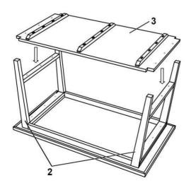
STEP# 4: Tighten the bolts to lock shelf and legs as shown below
