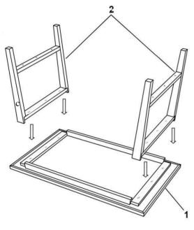
STEP# 2: Slightly tight the bolt and fully tight after completing step#3
