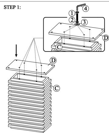
Step 1: Attach the Mounting Plate (D) to the Table Base (C) by inserting Allen Bolt (1), Lock Washer (2), Flat Washer (3) into the holes of the Table Base (C) and tighten by Allen Key (4).
