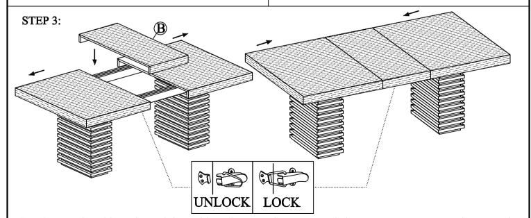
Step 3: Turn the table to the upright position. (\*Note: It is recommended to use two or more people to turn the table). Unlock the latch underneath the Table Top (A), and pull the Table Top (A) from both ends. Inserting the Table Leaf (B) in the middle of Table Top (A), close the Table Top (A) by pushing from both ends. Lock the latch underneath the Table Top (A) to prevent from sliding. Assembly of product is now completed.
