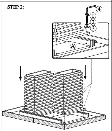
Step 2: Place the Table Top (A) upside down on the floor with a piece of cloth or carpet to prevent finish from scratching. Attach the assembly Table Base (C) in Step 1 to the Table Top (A) by inserting Allen Bolt (1), Lock Washer (2), Flat Washer (3) and tighten by Allen Key (4).
