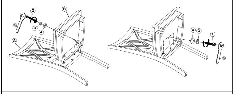
**STEP 2**: Attach Front Leg (C) to Seat Cushion w/ Seat Box (B) by using Flat Washer (4), Lock Washer (3) and Hex Nut (5), secure by Wrench (6). Fully tighten all bolts and screws as this time. Assembly product is now completed.
