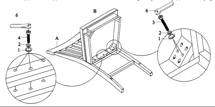
Step 2: Attach the LSF/RSF Front Leg (C) to the Seat Box w/ Seat Panel (B) by using Spring Washer (1), Flat Washer (2), Hex Nut (5) and Wrench (6). Then insert Front Stretcher (D), LSF/RSF Stretcher (E) into holes on legs and secure with Screw (7) and Philip Screwdriver (not provided). Fully tighten all screws and hex nuts, turn the chair to upright position. Product assembly is now completed.
