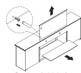
(Remove the screws from the back panel)
