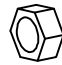
x8 Hex nut Ø5/16"x6mm * x8 Écrou hexagonal Ø5/16"x6mm x8 Tuerca hexagonal Ø5/16"6mm
