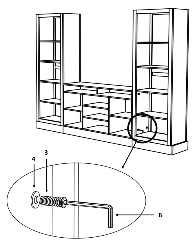
NOTE: FIRST TIGHTEN THE BOLTS HALF-WAY, THEN DOUBLE CHECK THAT EVERYTHING IS ALIGNED. ONCE EVERYTHING IS ALIGNED, PROCEED WITH TIGHTENING THE BOLTS FULLY.
