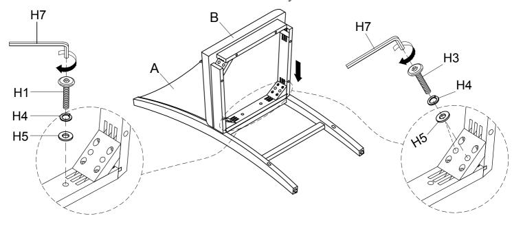
STEP 2 (x2) Do not over-tighten the bolts. Make sure you use the lock washers to ensure the bolts stay fastened.
