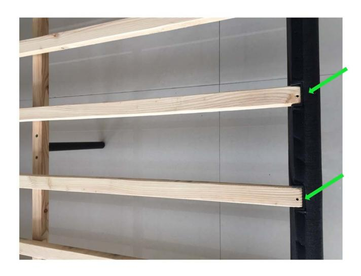
Use a Phillips (star head) screw driver to attach the 2 middle slats to the side frames using the wood screws (R)
