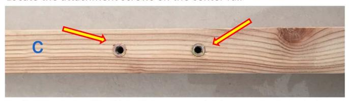
Attach the support leg (J) to the center rail (C) using the bolts (M) and washers (N). **VERY IMPORTANT**, the bolts must be attached from the opposite side of where the attachment nut is flush against the rail.
