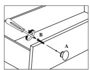
Remove the wooden knob and change to metal knob handle.
