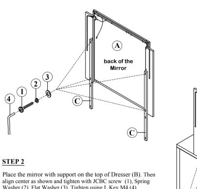
Place the mirror with support on the top of Dresser (B). Then align center as shown and tighten with JCBC screw (1), Spring Washer (2), Flat Washer (3). Tighten using L Key M4 (4).
