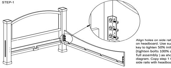
Align holes on side rail with holes on headboard. Use supplied allen key to tighten 50% initially (tighten bolts 100% after doing full assembly ) as shown in diagram. Copy step 1 for other side rails with headboard
