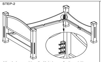
Align holes on side rail with holes on footboard. Use supplied allen key to tighten 50% initially (tighten bolts 100% after doing full assembly ) as shown in diagram. Copy step 2 for other side rails with footboard
