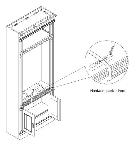
For your safety, once wall is fully assembled, secure to wall Wall Strap E.
