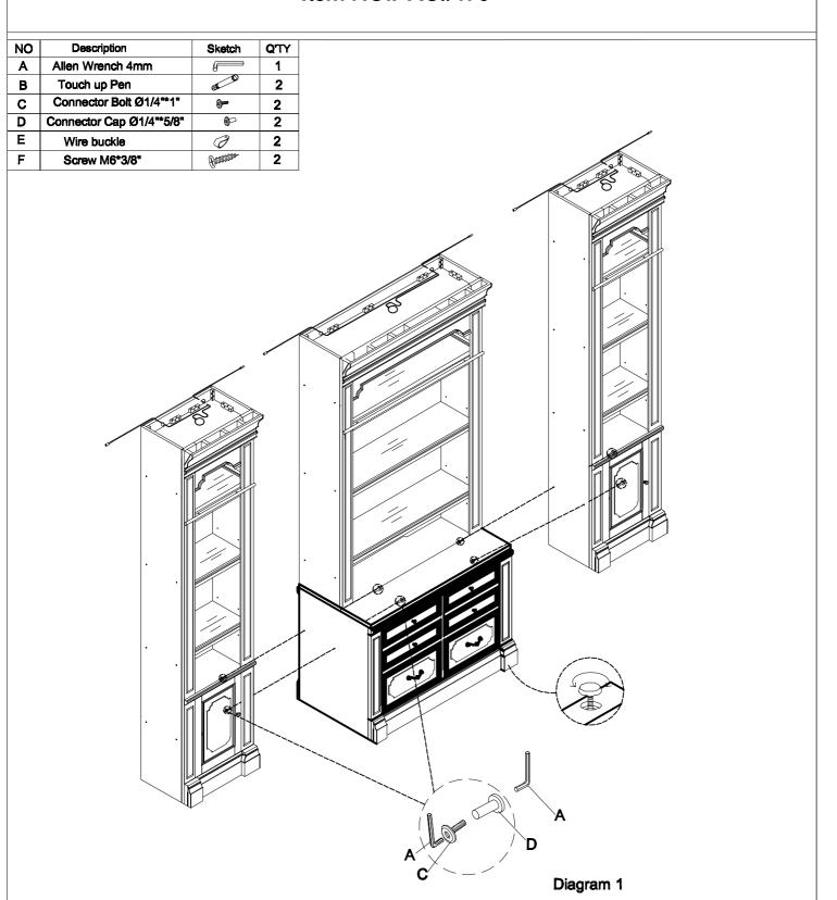
Align and connect cabinets with Connector Bolt C and Connector Cap D. See Diagram 1.
