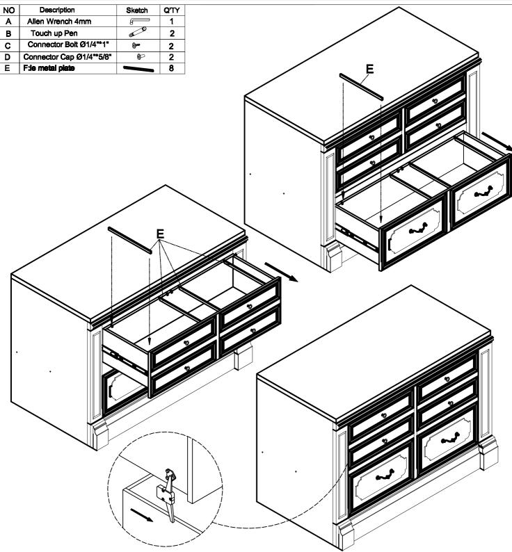
This furniture is equipped with safety hardware to prevent both drawers from being opened at the same time, to prevent the cabinet from tipping forward. Please do not try to override this feature and completely close one drawer before opening the other.
