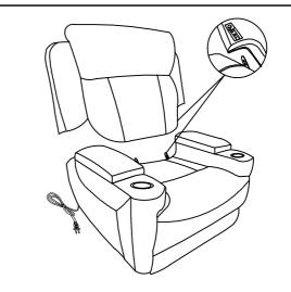
Connect wire behind seat to wire under the headrest, then slide back onto connecting brackets and push until you hear a clicking sound.
