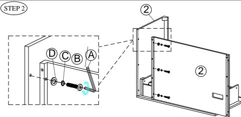
Step 2: Connect back panel and left side panel by using bolts (B), lock washers (C), & flat washers (D) with allen wrench (A) as shown in the illustration to the left.
