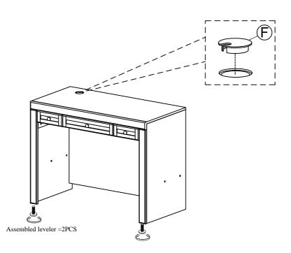
Step 5: Carefully turn the fully assembled Desk upright. Insert Wire Grommet (F) into wire hole on desk's top.
