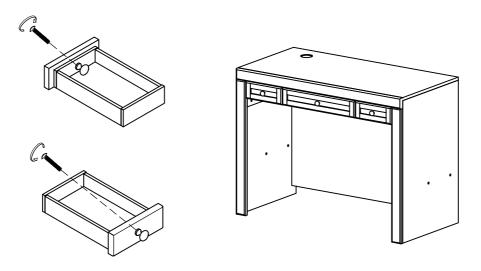
Open the pullout drawer, take off the handle & knobs installed on the back of drawer front and reattach the handle on the front side as shown.
