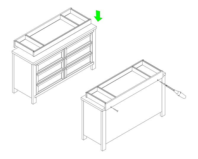
B. Insert the screws into the back of the changing topper and dresser, tighten with Screw driver. Check to see that the changing topper is secure.
