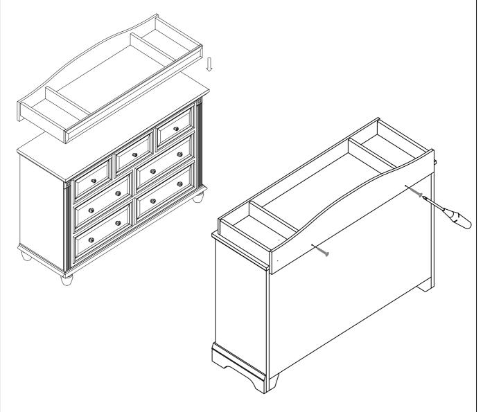
B. Insert the screws into the back of the changing topper and dresser, tighten with Screw driver. Check to see that the changing topper is secure.
