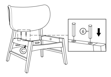
STEP 7: Place the Cushion Seat (F) upside down on a elevated surface (ex. Table top). Then, place the chair frame upside down and push the wood dowels (6) on the LSF Frame (C) into the holes on the bottom Cushion Seat (F).
