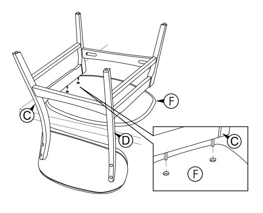
STEP 8: Assemble the chair frames (C&D) to the Cushion Seat (F) by using a screwdriver with hardware (4) & (5).
