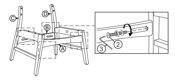
STEP 3: Assemble the Chair Back (E) to the top of the assembled chair frame by using the Allen Key (3) with the hardware (1).
