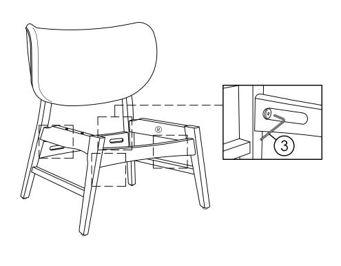
STEP 6: Insert Wood Dowel (6) into the designated hole on LSF Frame (C).
