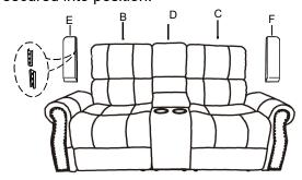
STEP 2:Install the LSF backrest (B), Console back (D), and RSF backrest (C) by align and insert the metal bracket to the metal brackests of the seat (A).Please make sure the brackets and console back are inserted all the way and secured intoposition.
