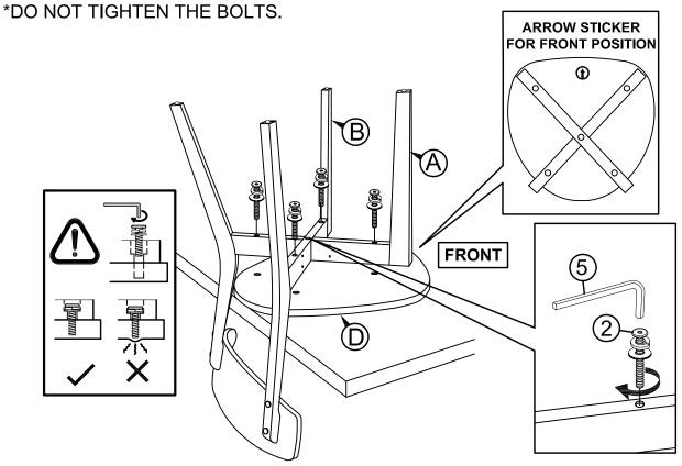
STEP 4: Next assemble the frame (A & B) to seat panel (D) by using Allen Key (5) with hardware 3 in the center hole of the frame.
