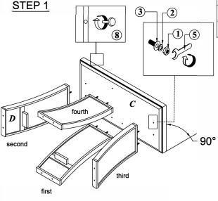
Flip over the table base & align the shelf panel to support leg by using csk screw as per diagram shown.
