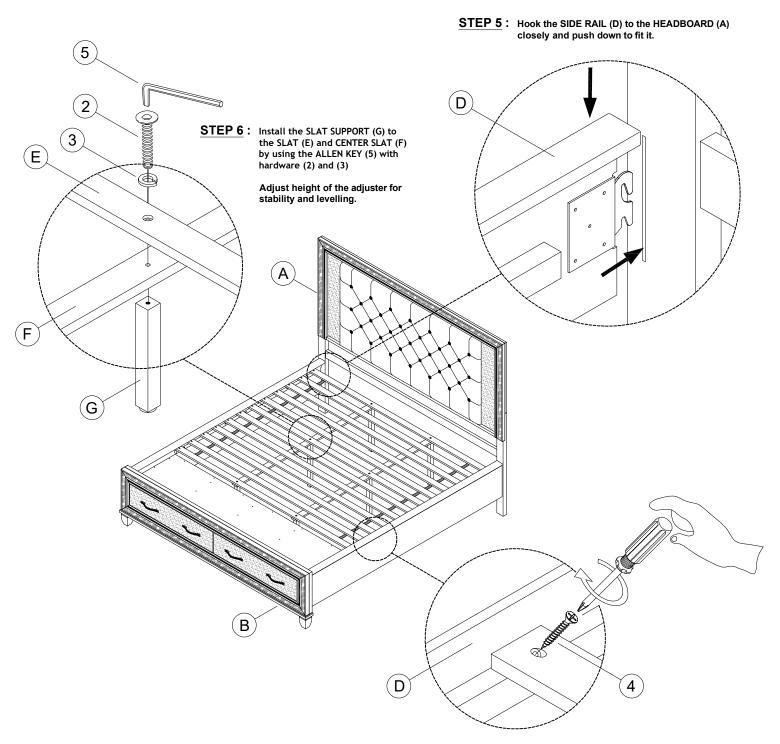
STEP 7: Install the SLAT (E) to the SIDE RAIL (D) by using the screwdriver and CSK SCREW (4).
