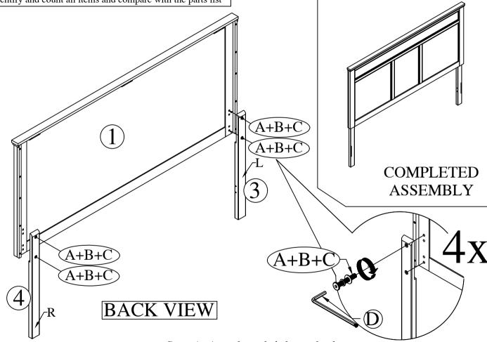
Step 1: Attach and tighten the leg posts (3 & 4) to the head board (1) by inserting JCBB bolt (A) with washers (B & C).
