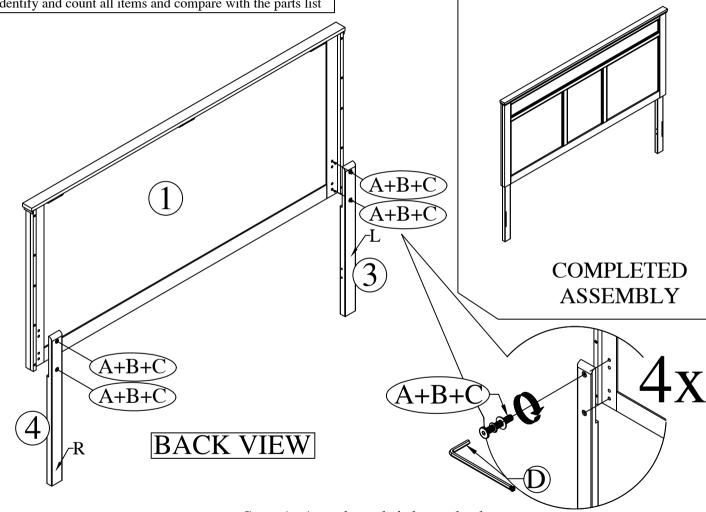
Step 1: Attach and tighten the leg posts (3 & 4) to the head board (1) by inserting JCBB bolt (A) with washers (B & C).
