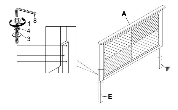
STEP 2 Assemble Headboard Crossbar (D) to HB legs (E) and (F) by using Allen Key (8) with hardware 1, 3, and 4.
