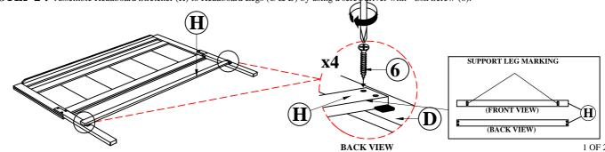
STEP 3: Hook side rail (G) to Headboard legs (C & D) and push it down to fit. Repeat with the other end of rail to hook onto Footboard (B). Tighten the 4 corners with Allen Key (5)
