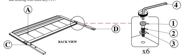
STEP 2: Assemble Headboard Stretcher (H) to Headboard Legs (C & D) by using a screwdriver with Csk Screw (6).
