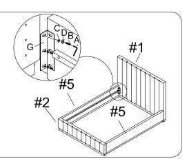
Step 2. Attach Wood strip for Side rail (#3) to side rail (#5) with Bolt (B), Lock washer (D) and
