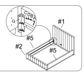
Step 2. Attach Wood strip for Side rail (#3) to side rail (#5) with Bolt (B), Lock washer (D) and Flat washer (C) .Tighten with Allen Key (A).
