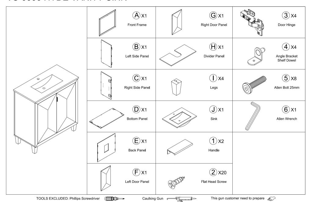
Step 1. Attach the legs (I) to the bottom panel (D) by using the Allen bolts 25mm (5) and the Allen wrench (6).
